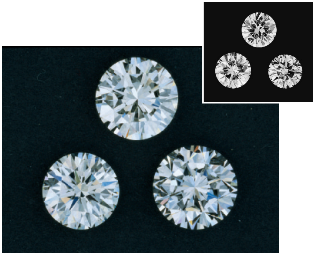
Figure 1. These round-brilliant-cut diamonds illustrate how cut affects face-up appearance. Of the three larger stones (1.07–1.50 ct), the one on the lower right (F color) is obviously less bright than the other two (above, H color, and lower left, E color). All three 0.35–0.38 ct diamonds in the inset are brighter, on average; but the F-color diamond on the lower right, which could be marketed as an “Ideal” cut, is less bright than the F- and G-color stones with larger tables and small crown angles. See table 1 for the proportions and other data on these diamonds. Photo © GIA and Tino Hammid.
